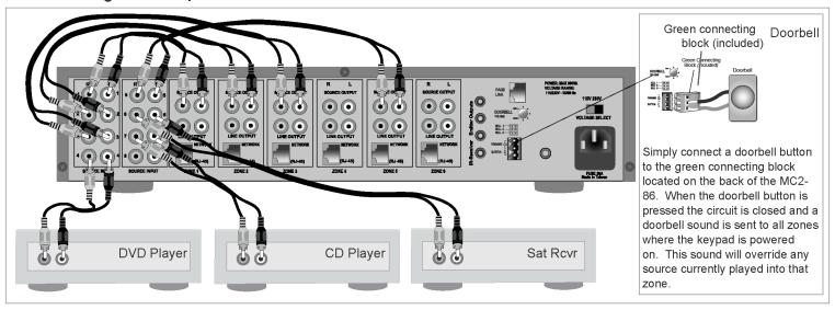
The MC2-86 allows you to select from up to 8 audio components, including up to 6 located throughout your home. In order to make use of an audio component located within a zone, including an audio component connected to the 3.5mm (1/8") input jack on a keypad, on the back of the MC2-86 you must connect the Source Output for that zone into one of the Source Inputs. We include six 1' shielded stereo patch cables for this purpose.
