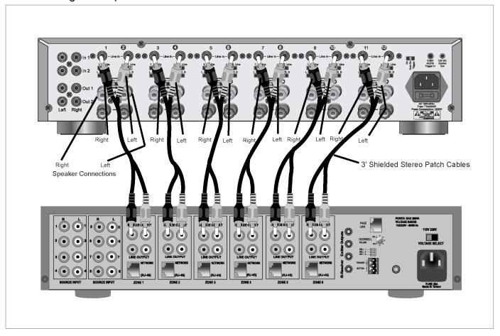
Use the Line Outputs on the MC2-86 to connect to the Line Inputs on the amplifiers for each zone. We include six 3' shielded stereo patch cables with the MC2-86 for this purpose. The diagram above shows the recommended connection to our DMA-1240 12-channel amplifier.
