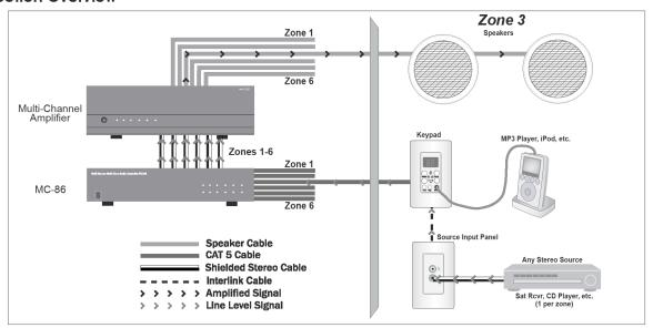
Think of the MC2-86 as the brain of the system. Based on information received from the keypads, it determines what source to play into each zone and the volume level to be sent to the amplifier.
