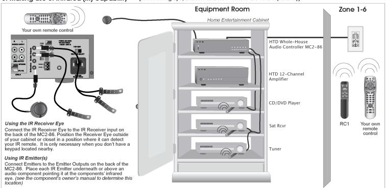
The MC2-86 is capable of passing infrared signals to other components positioned near it. When an infrared remote control is aimed at a Keypad the signal is transmitted through the Cat5e cable to the MC2-86 and on to other components through the use of IR emitters. In this way, you can control these centralized components from within each zone.
