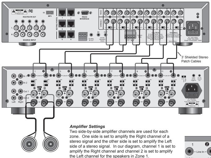
Level: Turn the rotary Level knob all the way clockwise to get the maximum power out of the amplifier. You can set the Level at less than maximum to limit the volume output in a zone (e.g. limit how loud a child can play his/her music). See "Best Practices" under Level Settings on Page 4 for more information.
