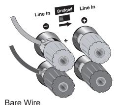
Rotate binding post counter-clockwise to reveal post. Strip back 3/8" insulation from cable. Tightly twist copper wires and wrap around post as shown. Rotate binding post clock-wise to tighten.
