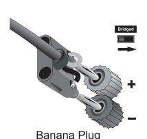
Make sure binding posts are tightened then push in banana plug
