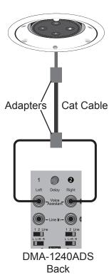
If you have a Cat 5/6 cable run but prefer to simply place the VAD on a counter or bookshelf rather than installing it in the wall or ceiling, you can power the VAD with its included power supply and purchase a set of audio adapters separately (see diagram to the right).
