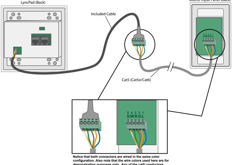
demonstration purposes only. Any of the cat5 conductors can be used as long as the connectors are wired identically. Lastly, notice that the connectors here are oriented to emphasize correct conductor placement.
