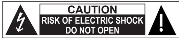
The lightning flash with arrowhead symbol, within an equilateral triangle, is intended to alert the user to the presence of un-insulated dangerous voltage within the product's enclosure that may be of sufficient magnitude to constitute a risk of electrical shock to persons.
