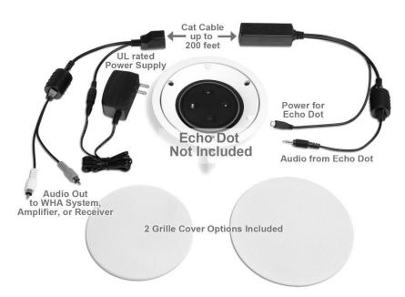
Ceiling / Wall Mount bracket with custom gasket that securely holds the Amazon Echo Dot (Gen 1&2).
