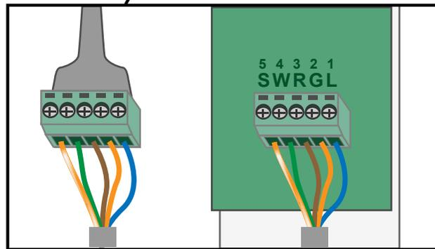
Notice that both connectors are wired in the same color configuration. Also note that the wire colors used here are for demonstration purposes only. Any of the cat5 conductors can be used as long as the connectors are wired identically. Lastly, notice that the connectors here are oriented to emphasize correct conductor placement.
